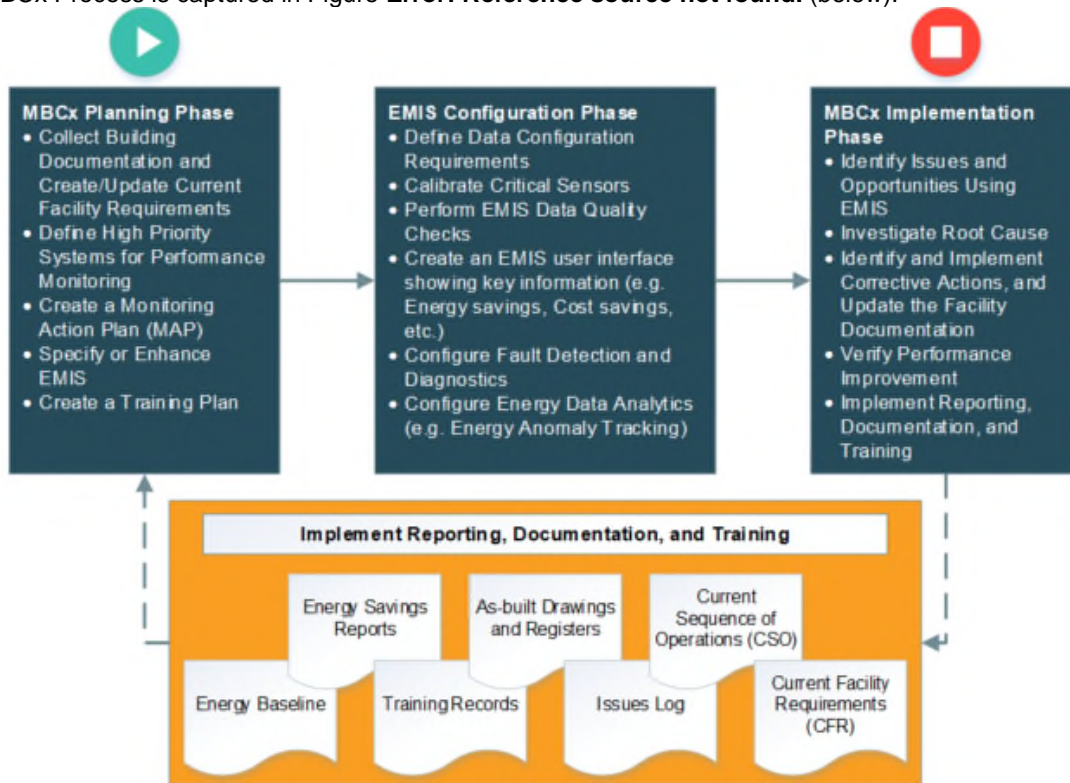
Figure 23: Monitoring-based Commissioning (MBCx) Process
